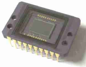
Monochrome, Progressive Scan 2/3"-CCD Image Sensor Sony ICX285AL
